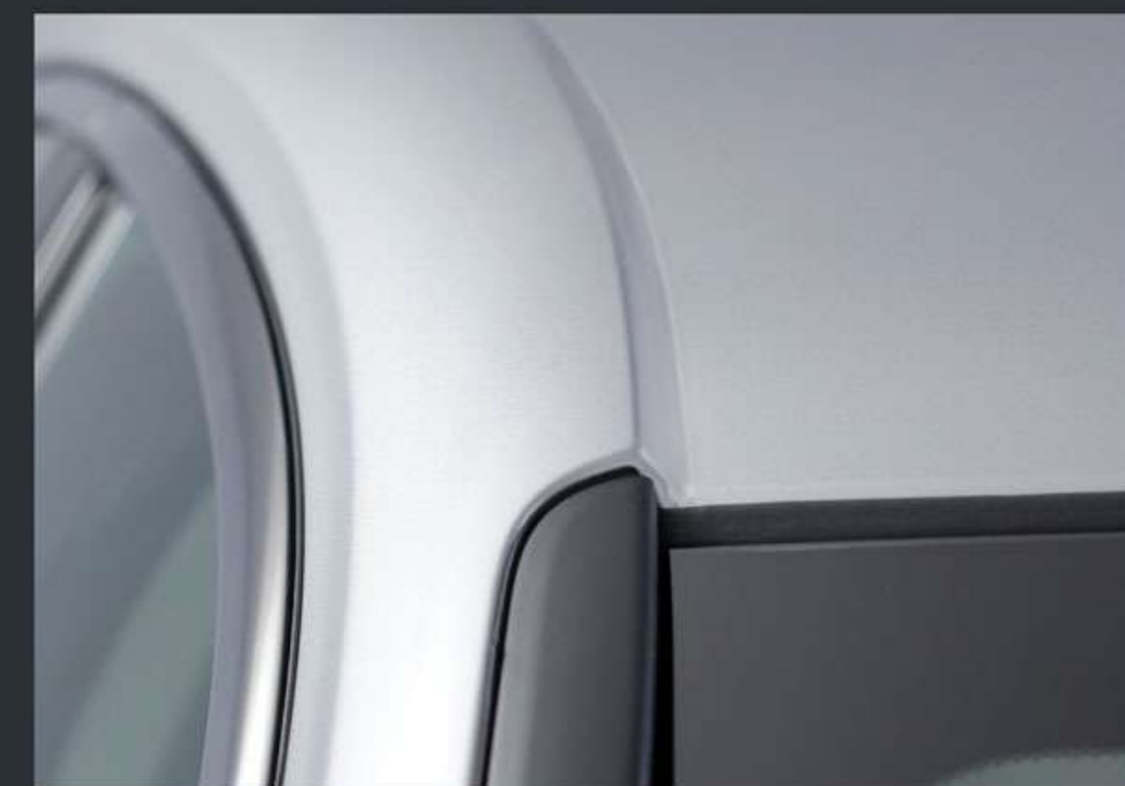
LAZER BRAZED ROOF (NOISELESS ROOF): Realization of the sleek design by applying brazing to the roof.
