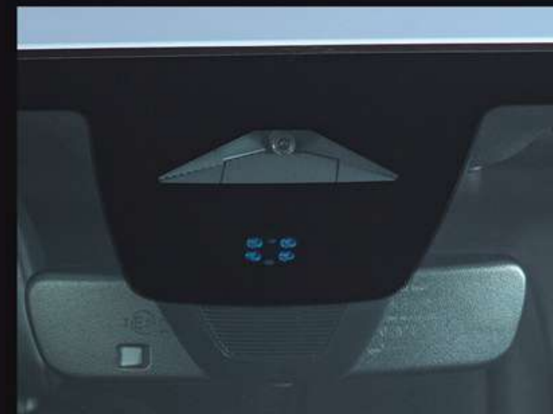
RAIN SENSOR: Automatically activate wipers.
