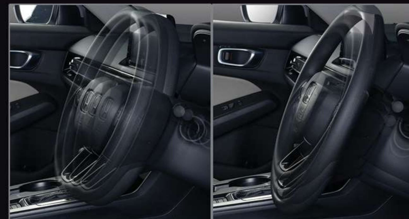
TILT & TELESCOPIC STEERING: Helps to adjust the steering wheel according to the driver's height by moving the wheel through tilted and telescopic movement.
